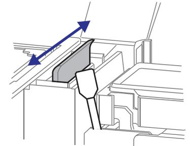
4 Use the cleaning stick to remove the ink and dust on the circumference of the cap.
